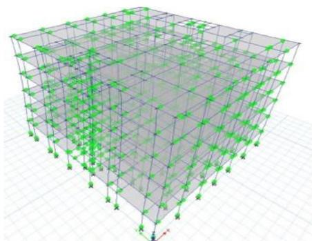
**Fig. 1 Without Infill Wall**
